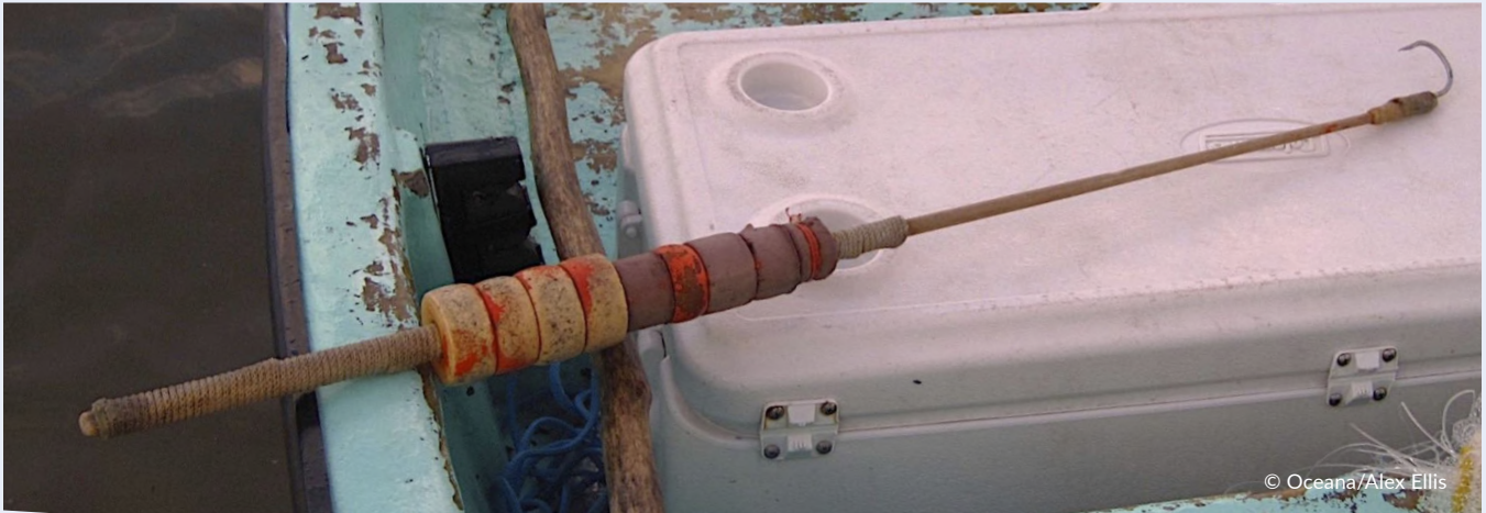
Figure 20. Hook stick modified with floats and used to pull fish in off a line. Hook sticks that are used to catch lobster do not have the floats on the end.
